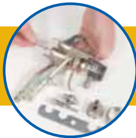
Easily remove needle assembly
