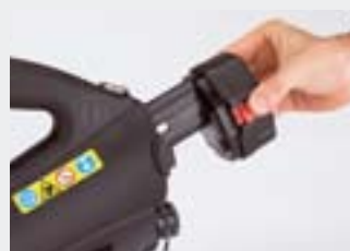
Operating and pressure release buttons mechanically interlocked
