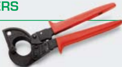
KT 3 For cutting cables \varnothing max 32 mm Weight: 0,59 kg Length: 255 mm
